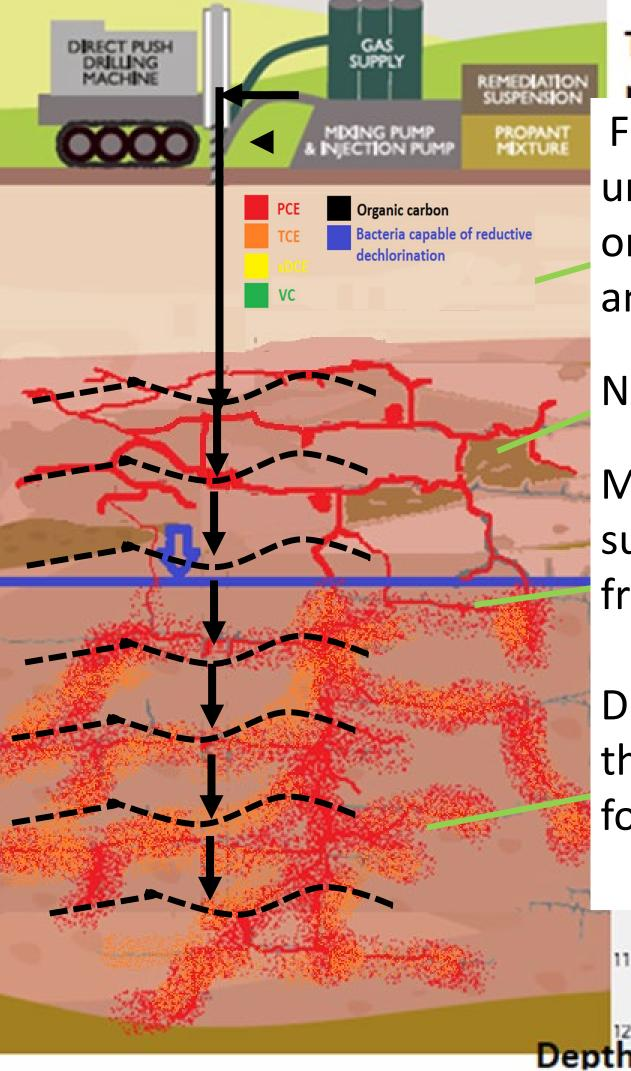
Conceptual site model Typical MIP profile (XSD) Frac In injections in to both unsaturated and saturated zone in order to widen current fracture system and fill it with reactive materials
