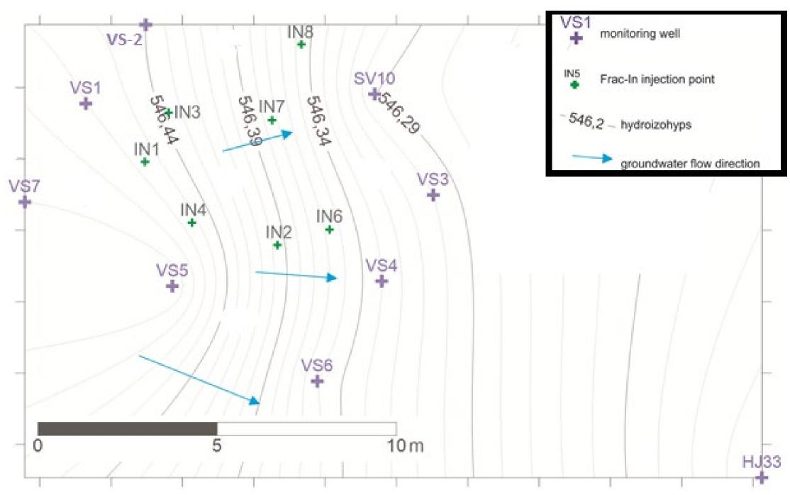
Pilot spot selected and monitoring system (consisting of 9 wells) installed based on previous MIP • survey and other works
